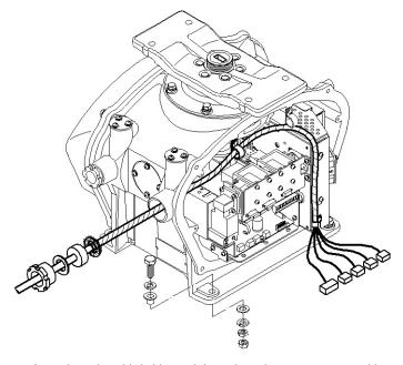
6. Screw down the cable holders and clips to keep the interconnection cable in place inside the scanner. The interconnection cable must be clumped at the copper tape at location A.
